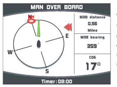
This page is shown when the Man Over Board function has been triggered. The **dead reckoned** distance and bearing to the man over board are displayed together with the boat's course over ground. The timer is triggered to give the time from event.
