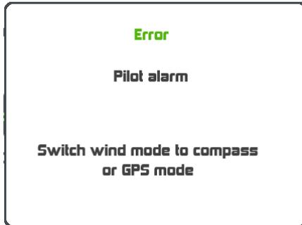
With the pilot in wind mode when an alarm has been set and the apparent wind angle is over the defined range. Press any key to inhibit the alarm for 7 minutes
