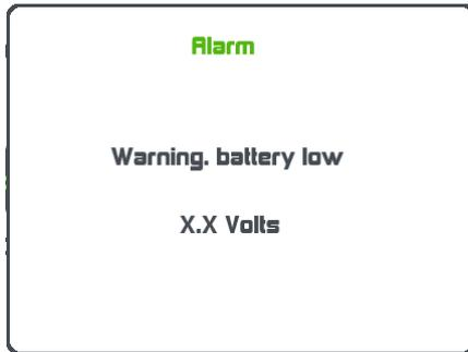
This message displays when the power supply to the Topline bus is below 9 Volts. Data is saved and the system switches off. Check the battery level and eventually charge it.
