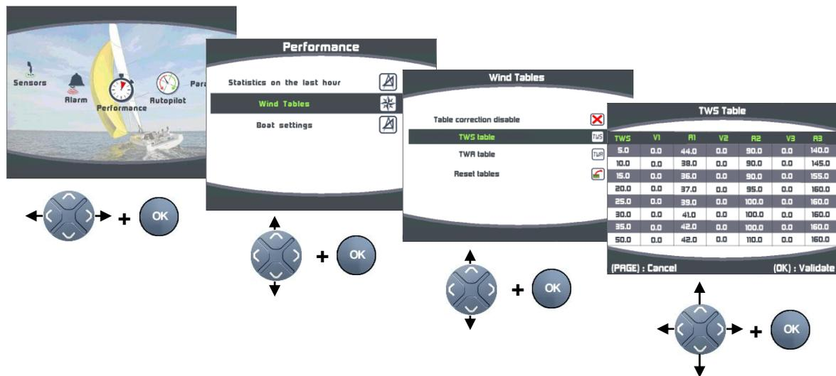
The column on the left indicates the true wind speed in knots, the “V1” column is the correction to apply in degrees and the “A1” column indicates on which angle the correction will apply. The same pattern applies for “V2” and “A2” for sidewind and “V3” “A3” for downwind.
