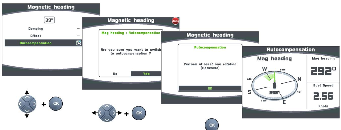
While swinging the **fluxgate**, or **Regatta** compass, you can display the Course Over Ground in a window to show the progress of the manoeuvre. In the case of the **Regatta** compass without COG data on the bus the progression will not be displayed and you will need to follow the procedure from the bowl compass at the helm.
