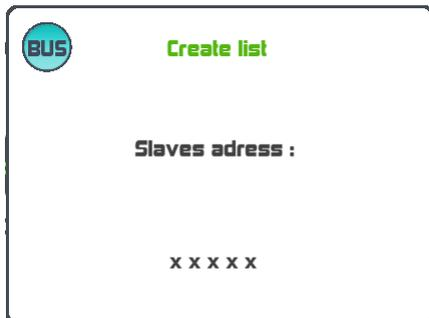
Multigraphic being set as “Master”, when the system creates the list (search all sensors and displays in the bus), it displays addresses for slave displays.
