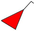
The red targets are hazardous vessels that are inside the CPA and TCPA limits you have set. The front arrow represents the vessels movement.
