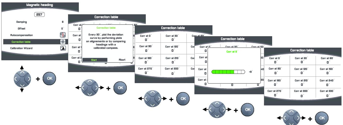
When this table is completed your compass is corrected for the deviation curve.
