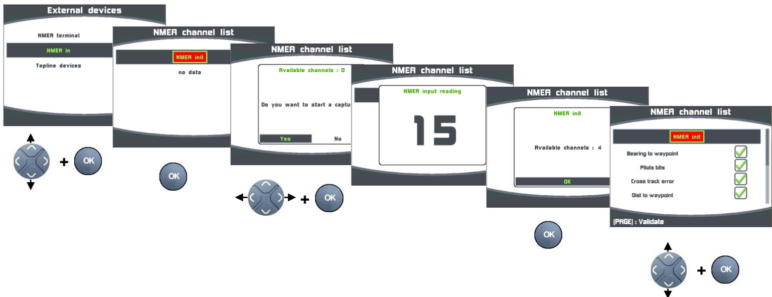
All NMEA channels are activated by default. You can choose to inhibit some channels. This is done by selecting the chosen channel and pressing .
