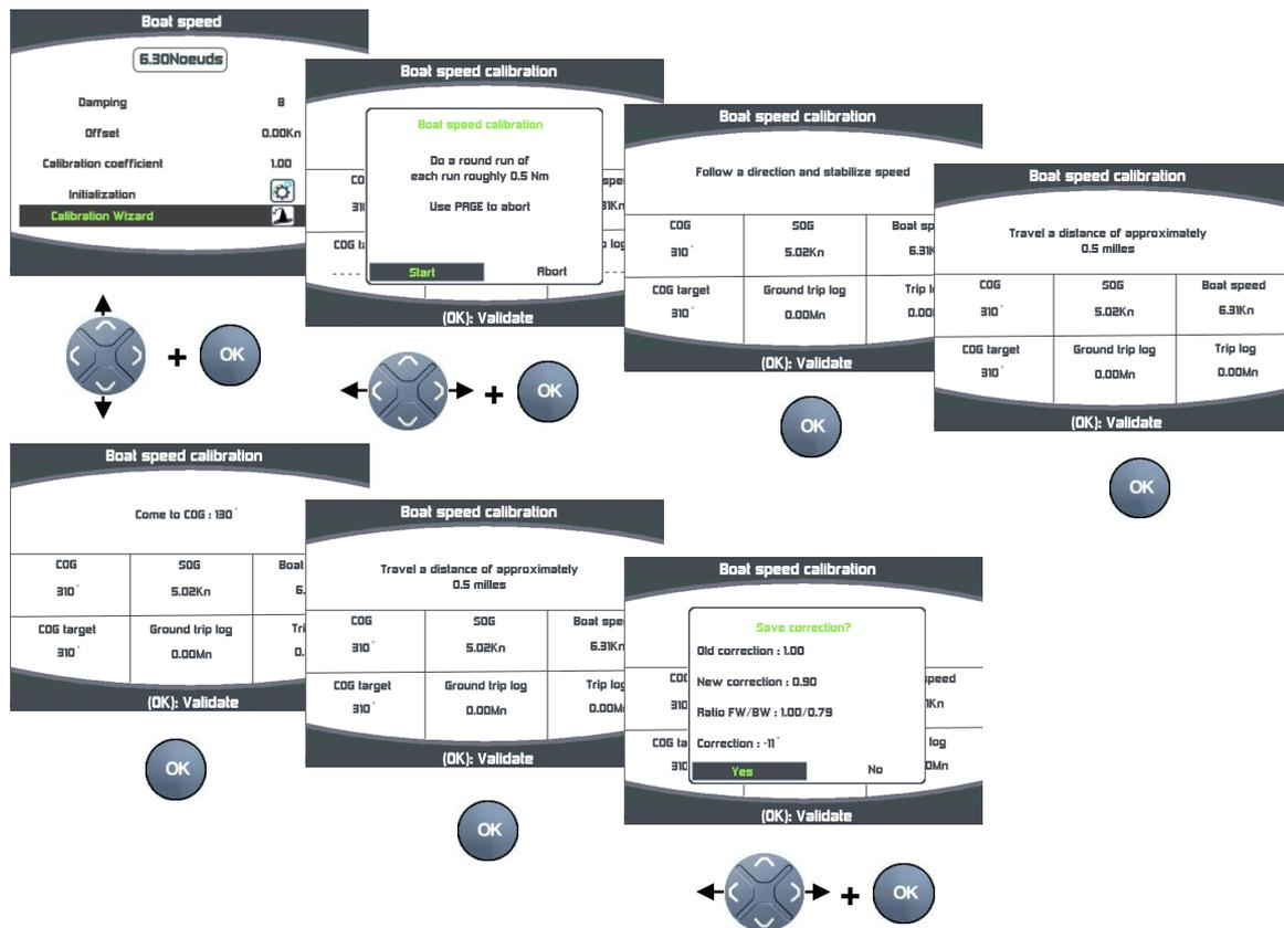
This page displays the current calibration value (old correction), the new calibration value (new correction), the factors calculated from the runs (ratio FW/BW) and the correction factor for boat speed.
