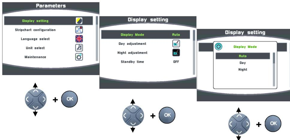
Auto: Backlighting toggles automatically between Night and Day settings, driven by a light sensor. The Backlight intensity and the Skin are those set for each Mode.
