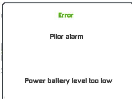
The battery powering the pilot's drive unit has reached a lower voltage than defined in the setup. Press any key to inhibit the alarm for 7 minutes.
